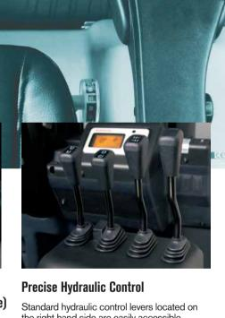
the right hand side are easily accessible. Combined with an excellently tuned hydraulic system, materials-handling activities can be performed with high accuracy.
